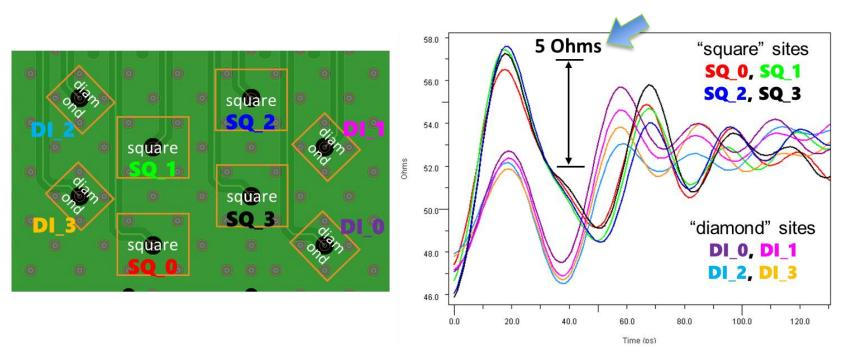
50 Ohm signal via misses by 5 Ohms, due to GRV config
