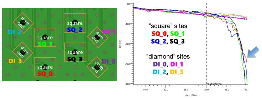
99% of "square" signals lost at 40 GHz – 100 mil via IL greater than 15" trace
