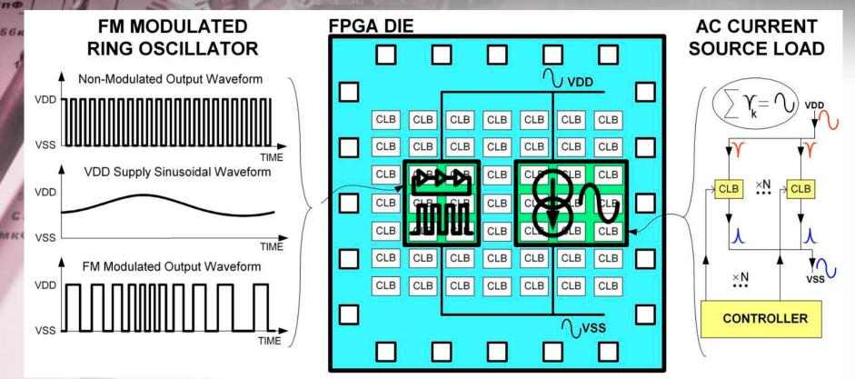
The sinusoidal current flows through the power distribution network and generates sinusoidal variation of the on-die power supply voltage
