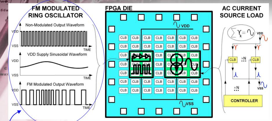
The sinusoidal variation of the voltage supply modulates the frequency of the ring oscillator
