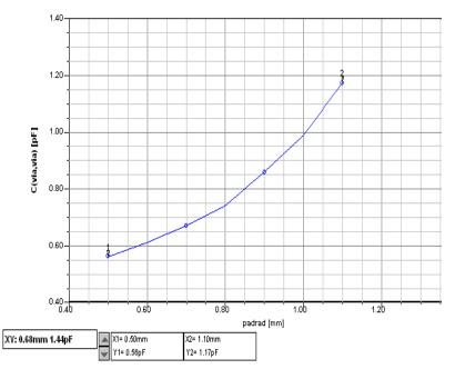
The graph shows a much stronger effect from the pad radius than the center barrel radius - the capacitance changes from 0.56 pF to 1.17 pF (100% variation) over the range of the sweep.
