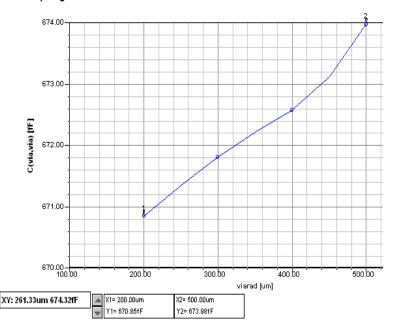
The graph shows that the via capacitance is only slightly affected by the radius of the center barrel: the change in capacitance is from
