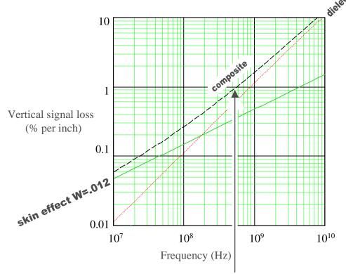
For more accurate results use a 2-D field solver to compute skin loss and effective dielectric loss tangent
