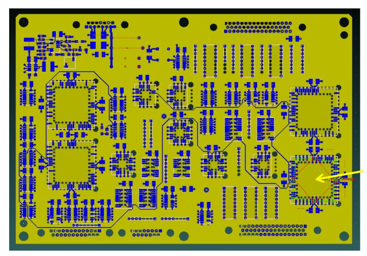
Measuring impedance at the six VCC pins on U41
