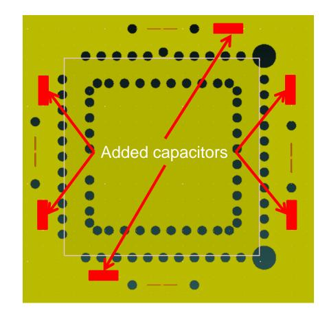
Six 8 nF capacitors were added near U41 to cancel resonance at 80 MHz
