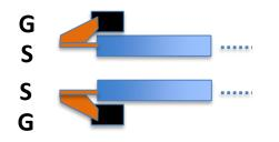
When the GND blade is "approximately" on the back, the ODD and EVEN (a) mode Insertion loss are by the same.
