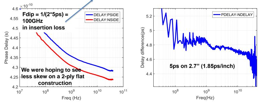
More likely to find high delta delay [ps/inch] values on shorter traces. On longer traces the normal meandering of the weave tends to statistically equalize the delay, although can't be guaranteed in the worst case
