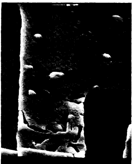
Fig. 1. One-mil wide Al stripe which has failed due to void formation by electromigration.
