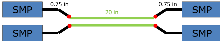
[100ohms, 21.5inch-long Differential Trace]
