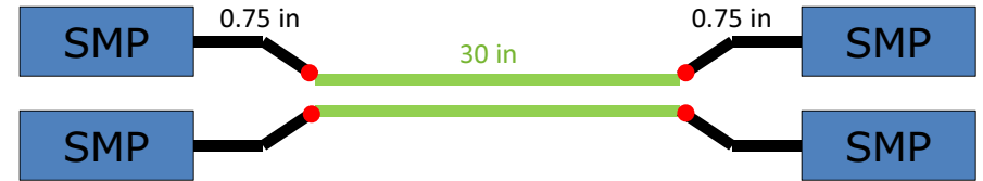
[100ohms, 31.5inch-long Differential Trace]
