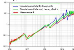
PDN's Input impedance profile including the effects from PCB/pkg/chip
