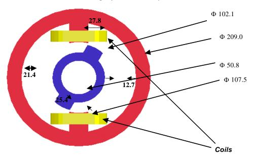
Axial length (rotor and stator) = 25.4
